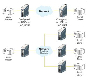
Each product passes data from its serial interface to the serial interface of the other product. This enables long distance serial communication using preexisting networks.
