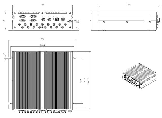
Figure 5 **Dimensions of the Housing**
