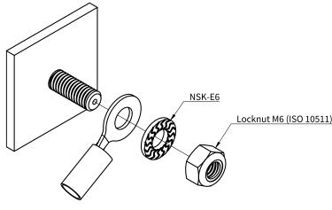
Figure 6 Earth Cable Mounting on Earth Stud
