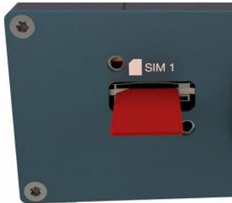
Figure 6: Inserting SIM card into SIM1 slot
