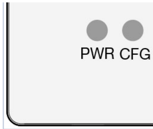
Figure 6: The Power and Config LEDs on the Merlin router
