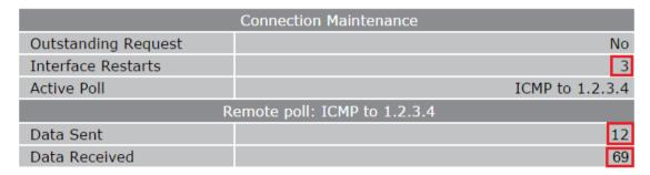
The *Interface Restarts* shows how often the interface has been restarted due to failed responses to the monitoring pings. This page also shows how many pings have been transmitted (Data sent) and how many replies have been received (Data Received).
