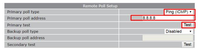
**NB:** Set up the **backup poll type** and **address** if you want to send test pings to a second IP address should pings to the primary IP address fail.
