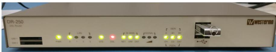
Once complete all LEDs will flash excluding the x3 Signal LEDs indicating the backup is complete.
