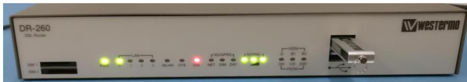
During backup only the x3 Signal LEDs will flash
