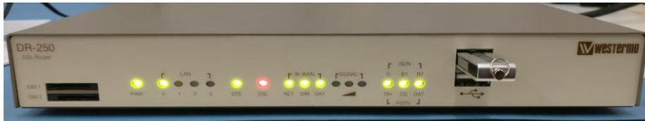
Once complete all LEDs will flash excluding the x3 Signal LEDs indicating the backup is complete. Power cycle the router and the upgrade is complete.
