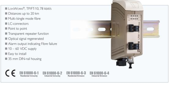
LONWORKS® to fibre optic link, point-to-point applications The LRW-102PP is a fibre optic modem designed for point-to-point fibre opticconnections between LONWORKS® networks.
