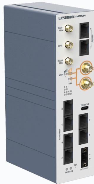
The Merlin 4600 series of versatile cellular routers provide high speed data network connectivity for demanding industrial and smart grid applications. Coupled with the Zero Touch Deployment software Activator, it provides cost-effective, reliable and consistent onboarding of routers in large-scale projects.
