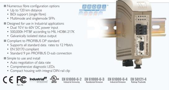
The ODW-610-F1 has been designed to allow the PROFIBUS DP protocol to be transmitted point to point over a fibre optic link. The design allows the use of a range of Westermo verified SFP (Small Form Pluggable) transceivers which can provide solutions with, for example, only a single fibre or distances up to 120 km.
