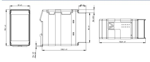
**Dimension W x H x D**  $55 \times 100 \times 132 \text{ mm} (2.16 \times 3.93 \times 5.19 \text{ in})$
