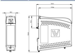
Dimension  $W \times H \times D$  $34 \times 123 \times 121 \text{ mm } (1.33 \times 4.84 \times 4.76 \text{ in})$
