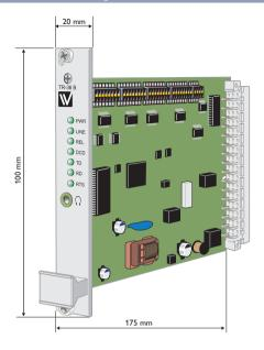
**Dimension W** x H x D  $20 \times 100 \times 175 \text{ mm } (0.78 \times 3.93 \times 6.88 \text{ in})$
