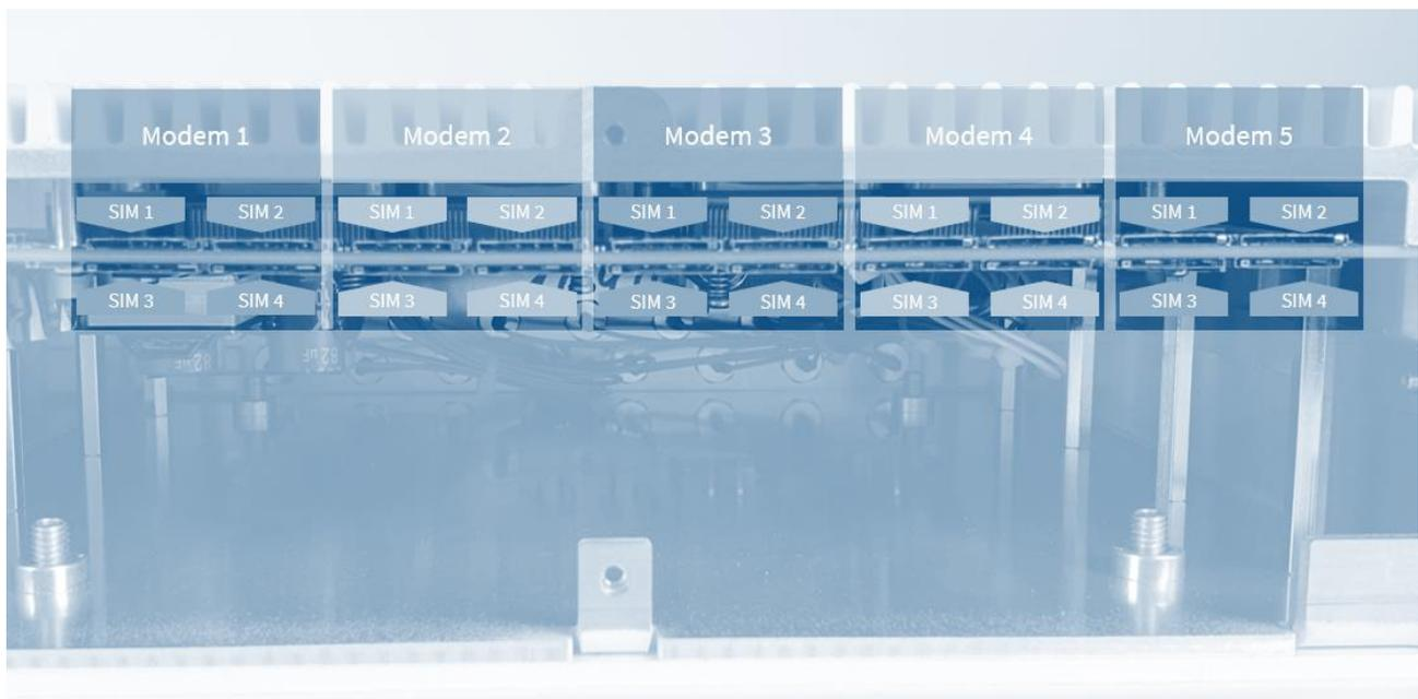
Figure 4 **SIM Slot Assignment per Modem**
