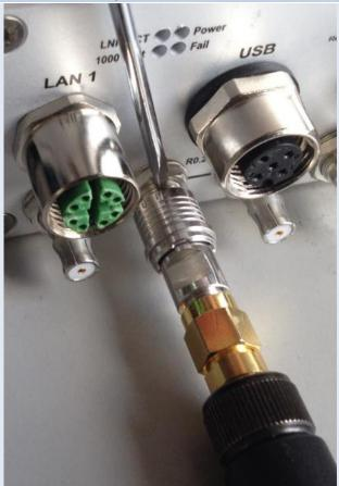
Rotate and/or push the screwdriver while pulling the antenna
