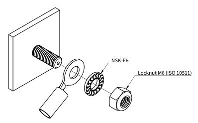
Figure 4 Earth Cable Mounting on Earth Stud
