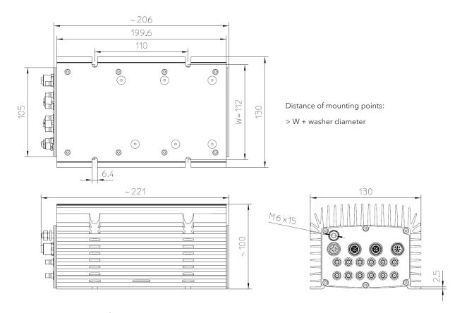
Figure 3 Dimensions of the Ibex-4000 Housing
