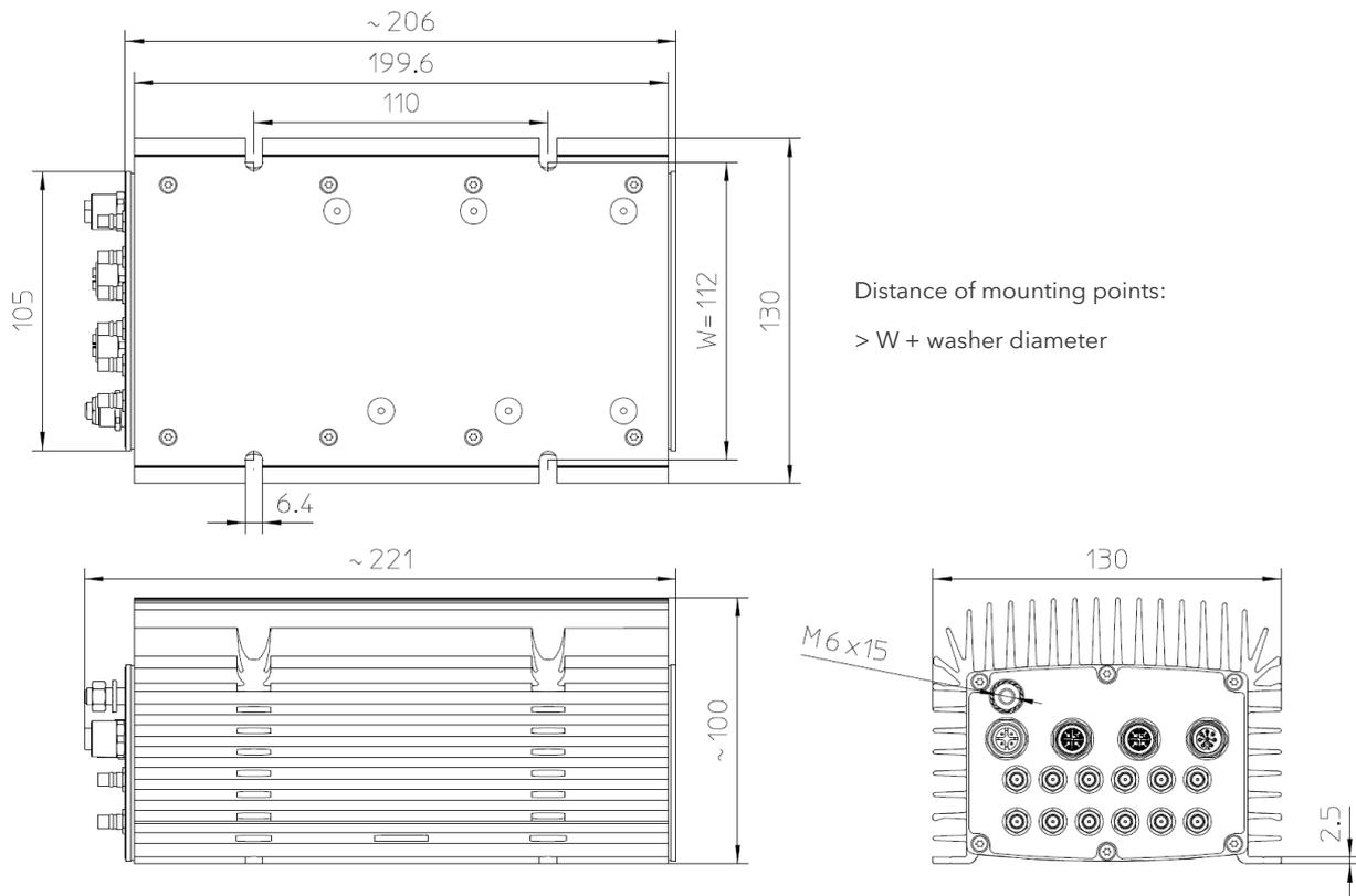
Figure 3 **Dimensions of the Ibex-4000 Housing**
