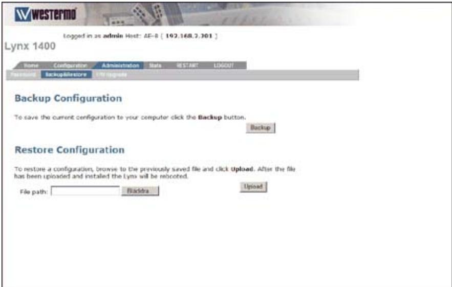
The configuration of the Lynx switch can be saved as a file to a PC. The file can then be used to restore the configuration later on, or used to configure another switch with identical configuration.
