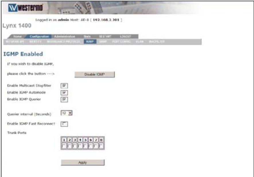
The Lynx switch supports IGMP (Internet Group Management Protocol) Snooping based on IGMP v1, IGMP v2 and IGMP v3. To enable IGMP Snooping, click *Enable IGMP*.
