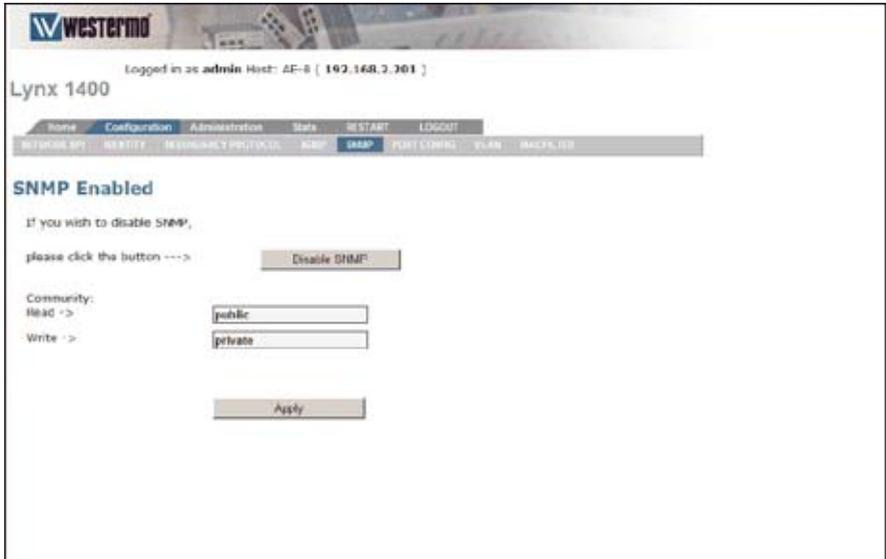
The Lynx has support for SNMP v2c with a range of MIBs, which are listed and explained in the Lynx White paper.
