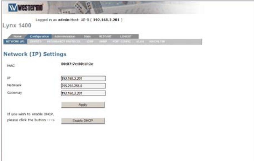
The Lynx switch IP-address can individually be changed via the Web Interface, another option is DHCP. These settings can be configured in the *Network (IP) Settings*.
