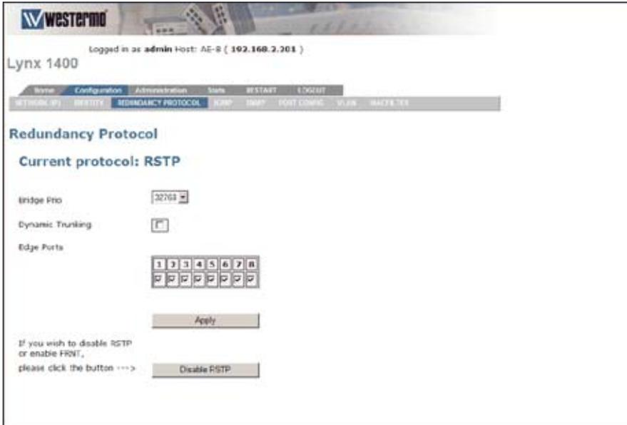
The Lynx switch support the Rapid Spanning Tree Protocol (RSTP) according to IEEE802.1w with fallback to the Spanning Tree Protocol (STP - IEEE802.1D). The STP fallback feature means that the Lynx switches can be used together with switches that only have support for STP.
