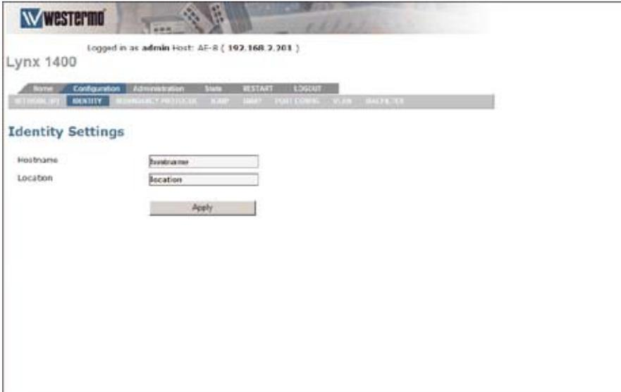
The Lynx switch identity can be changed via the Web Interface. These settings can be configured in the Identity Settings.
