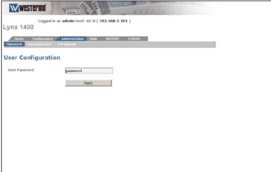
The Lynx switch administrator password can be changed via the Web Interface. These settings can be made in the *User Configuration*.
