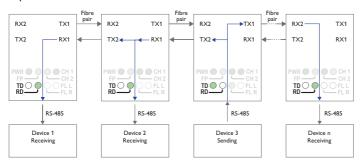
Data from some other communication device, for example device 3, is processed in the same way and sent out on both optical fibres TX1 and TX2.
