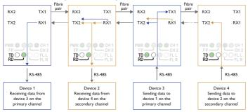
The fourth ODW-730 unit recieives data from communications device 4 on the RS-485 port and sends it out on optical fibre TX2 using the secondary data channel.
