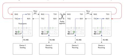
ODW-730 units located to the "right" side of the failure will send data in the opposite direction as before. Notice that still, it's only the first ODW-730 that is able to communicate in full duplex with other units, and that other units are incable of communicating with each other.
