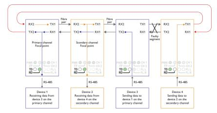
The other ODW-730 units will continue to send data out in as many directions as possible. Consequently, all communication devices will still be able to communicate with each other. Notice that the Ring Focal Points are now repeating incoming data from optical fibre RX2.
