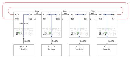
Data from comminication device 1 is received at the ODW-730 RS-485 port (as indicated by the TD LED), data bits are retimed according to the preset rate and sent out on the optical fibre TX1. The next ODW-730 unit receives data at optical fibre RX2 (as indicated by the RD LED), and data is sent out on the RS-485 port. Data is also repeated out on TX1 on to the next ODW-730 unit.
