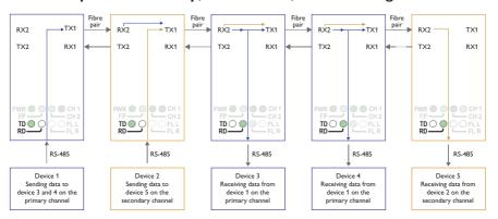
The first ODW-730 unit recieives data from communications device 1 on the RS-485 port and sends it out on optical fibre TX1 using the primary data channel.
