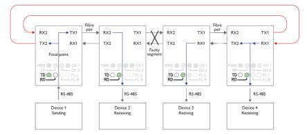
If an optical fibre segment fails, the ODW-730 Ring Focal Point will switch mode and start sending out data on both optical fibre ports, TX1 and TX2, simultaneously.
