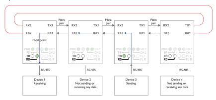
Data from some other communication device, for example device 3, is processed in the same way and sent out on optical fibre TX2. Intermediate ODW-730 units will receive this data at optical fibre RX1 and repeat it out on optical fibre TX2. But, intermediate units will not send any data received at RX1 on to the RS-485 port. **Only** the first ODW-730 (leftmost in the picture above) will have incomming data from optical fibre RX1 sent out on the RS-485 port.
