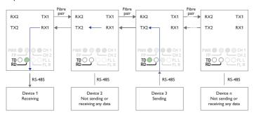
Data from some other communication device, for example device 3, is processed in the same way and sent out on optical fibre TX2. Intermediate ODW-730 units will receive this data at optical fibre RX1 and repeat it out on optical fibre TX2. But, intermediate units will not send any data received at RX1 on to the RS-485 port. Only the first ODW-730 (leftmost in the picture above) will have incomming data from optical fibre RX1 sent out on the RS-485 port.
