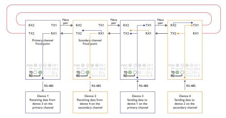
The fourth ODW-730 unit recieives data from communications device 4 on the RS-485 port and sends it out on both optical fibres TX1 and TX2 using the secondary data channel.
