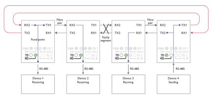
The other ODW-730 units will continue to send data out on both optical fibres TX1 and TX2. Consequently, all communication devices will still be able to communicate with each other. Notice that the Ring Focal Point is now repeating incoming data.
