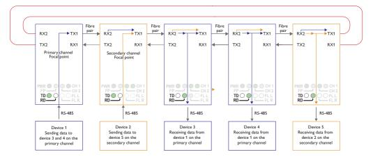
The first ODW-730 unit recieives data from communications device 1 on the RS-485 port and sends it out on optical fibre TX1 using the primary data channel.
