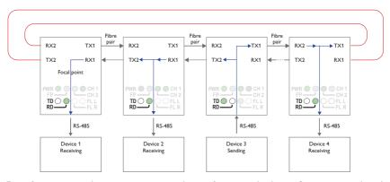
Data from some other communication device, for example device 3, is processed in the same way and sent out on both optical fibres TX1 and TX2. Notice that the Ring Focal point never repeats incoming data.
