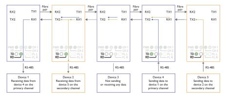
The fifth ODW-730 unit recieives data from communications device 5 on the RS-485 port and sends it out on optical fibre TX2 using the secondary data channel.
