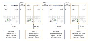
The first ODW-730 unit recieives data from communications device 1 on the RS-485 port and sends it out on optical fibre TX1 using the primary data channel.
