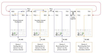
If an optical fibre segment fails, the ODW-730 Ring Focal Points will switch mode and start sending out data on both optical fibre ports, TX1 and TX2, simultaneously.
