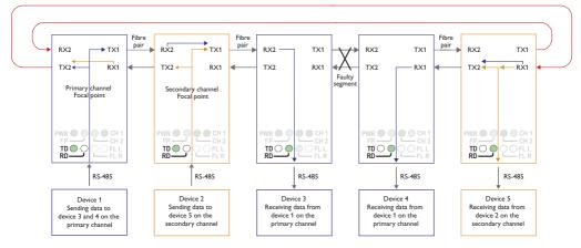
If an optical fibre segment fails, the ODW-730 Ring Focal Points will switch mode and start sending out data on both optical fibre ports, TX1 and TX2, simultaneously.
