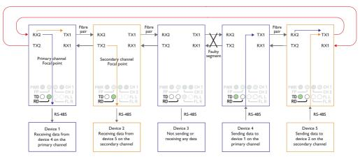
The third and fourth ODW-730 units will now switch direction so that data is sent out on optical fibre TX1 instead of TX2. (Not shown in the picture above, is that the third ODW will continue to send data out on TX2).
