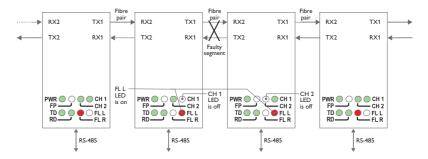
If an optical fibre segment fails, to determine wich fibre segment has failed, look at the FL L, FL R, CH 1 and CH 2 LED's as show in the picture above.
