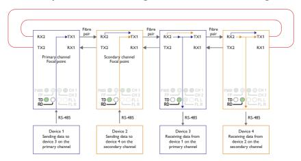
The first ODW-730 unit recieives data from communications device 1 on the RS-485 port and sends it out on optical fibre TX1 using the primary data channel.
