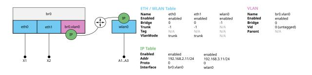
Figure 4.4: Client (STA) Network Configuration Example 1
