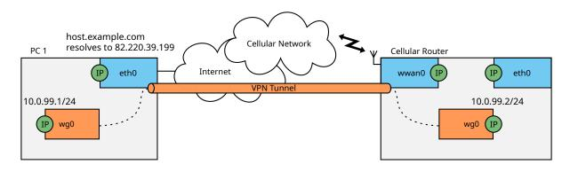
Figure 4.13: WireGuard FQDN Re-Resolving
