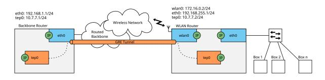
Figure 4.7: GRE in a Wireless Network
