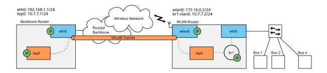
Figure 4.9: VXLAN in a Wireless Network
