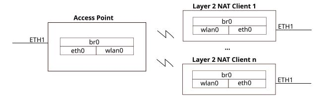
Figure 4.15: Layer 2 NAT bridge mode setup
