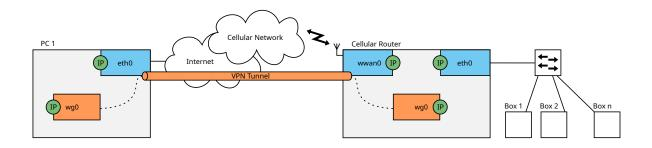
Figure 4.12: WireGuard in a Cellular Network
