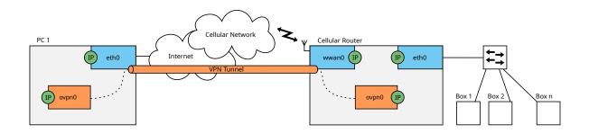
Figure 4.11: OpenVPN in a Cellular Network
