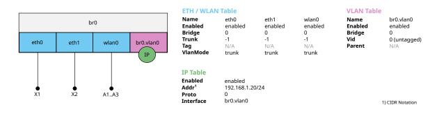
Figure 4.1: Access Point Network Configuration Example
