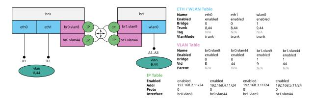
Figure 4.5: Client (STA) Network Configuration Example 2
