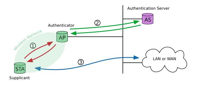
Figure 4.16: Supplicant authentication using IEEE 802.1X
