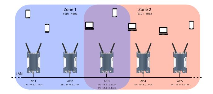
Figure 4.37: Spliting into Steering Zones
