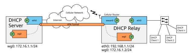
Figure 4.28: DHCP Relay From eth0 to a Central DHCP Server
