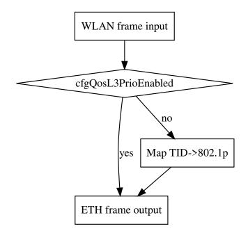
When L3 processing is disabled, the received TID will be mapped to the 802.1p field in the 802.1q tag.
