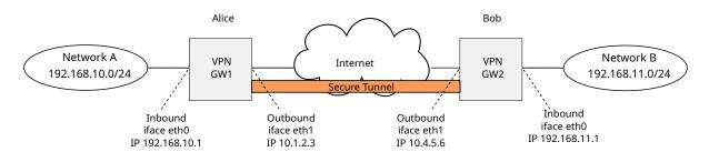
Figure 4.10: IPsec VPN Sample Topology
