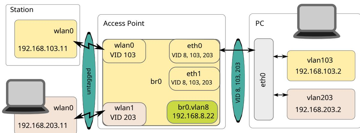
**Figure 4.27:** Multi SSID and VLAN example setup
