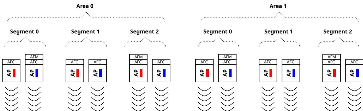
Figure 4.41: Area Frequency Management Principle
