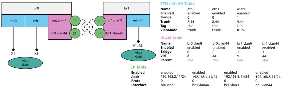
Figure 4.5: Client (STA) Network Configuration Example 2
