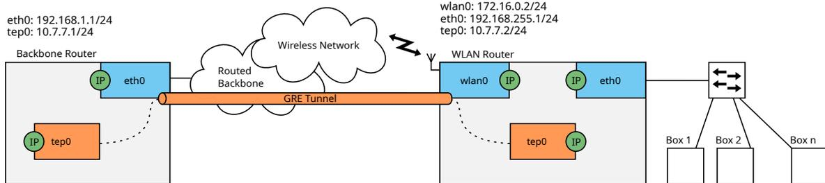
**Figure 4.7:** GRE in a Wireless Network
