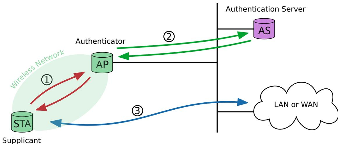
**Figure 4.16:** Supplicant authentication using IEEE 802.1X
