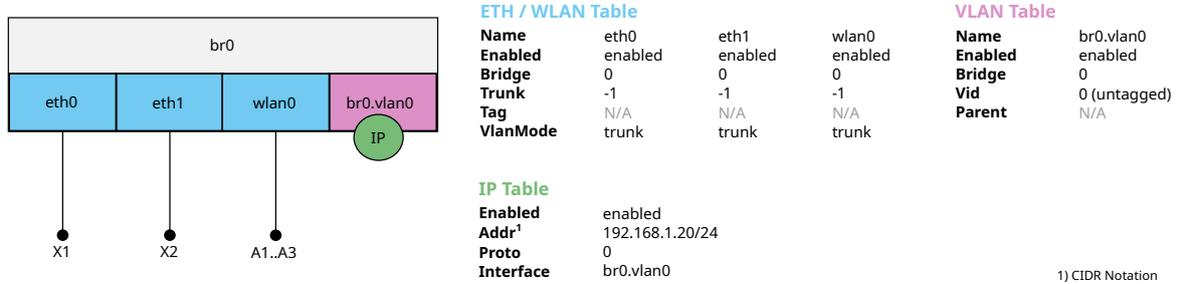
**Figure 4.1: Access Point Network Configuration Example**
