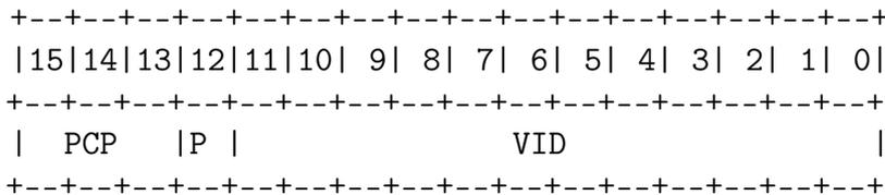
Bits 0-11 (VID) are the vlan number. Bit 12 (P) represents the existence of a vlan header. Bits 13-15 (PCP) are the vlan priority. The first part before the / is the value to match on. The second part after the / is the mask applied on the value. This can be used to match tagged or untagged frames, ranges of vlans or the priority.
