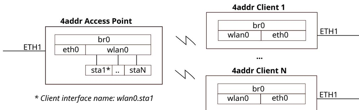
**Figure 4.14:** 4addr bridge mode setup
