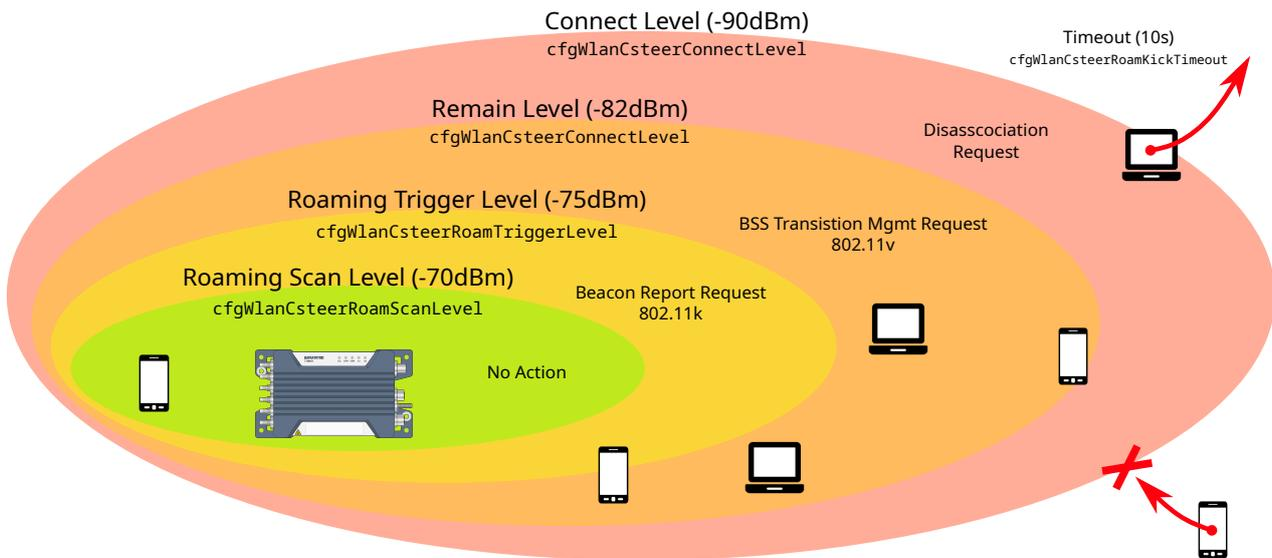
Figure 4.36: Client Steering Roaming Levels
