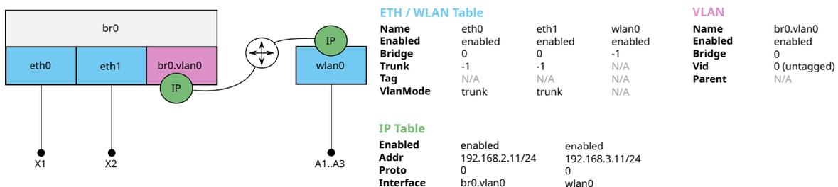
Figure 4.4: Client (STA) Network Configuration Example 1
