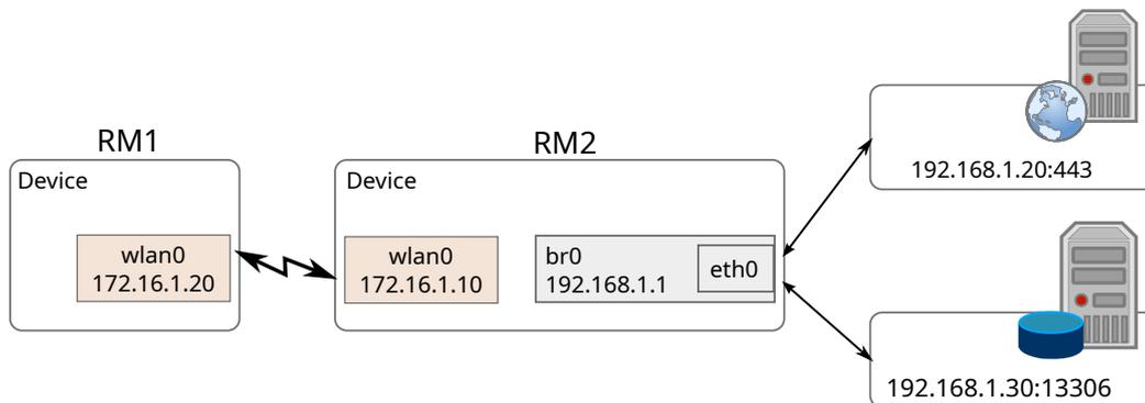
**Figure 4.44:** Port forward to servers behind an device
