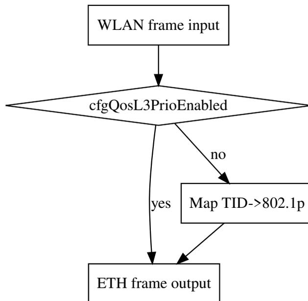
When L3 processing is disabled, the received TID will be mapped to the 802.1p field in the 802.1q tag.
