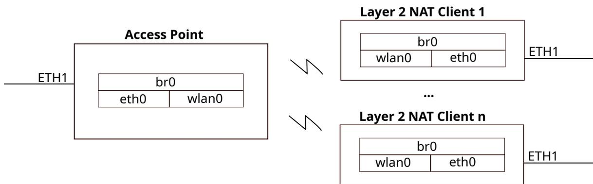
**Figure 4.15:** Layer 2 NAT bridge mode setup
