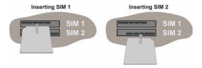
In both cases, the end of the SIM card with the chamfered corner should be inserted first. For SIM 1 the contacts should be face down. For SIM 2 the contacts should be face up. The easiest way to get started is to use SIM-cards without PIN-code. If the PIN-code is activated it is possible to set this up in the settings for the router.
