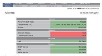
**Note:** If the unit is not yet configured it is likely that the Network Status and Connection Status will indicate a fault condition. This is normal.
