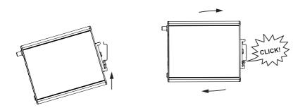
The MRD-315 and MRD-415 includes integrated mounting flanges and can be attached to a panel or tray by means of screws, using the slots provided. Alternatively the MRD-315 and MRD-415 can be DIN rail mounted, using the DIN rail mounting kit.
