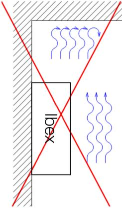
Figure 8. Installation with reduced natural convection airflow
