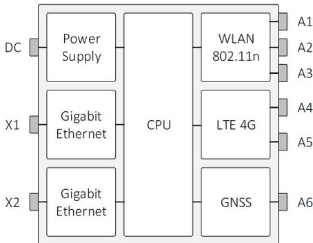
Figure 3. Ibex-RT-630-LV/Ibex-RT-630-HV block diagram
