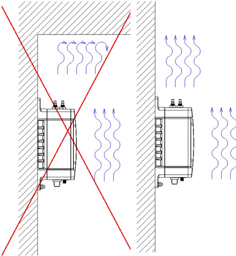
Figure 8. Installation with reduced natural convection airflow
