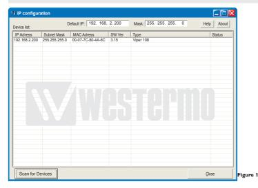
By clicking the "Scan for Devices" button the IP Configuration tool will detect the switches/routers in the network. The software will list all Westermo managed switches or routers connected to the network. Information as in the figure 1 will appear for each detected unit connected to the same network as your PC.
