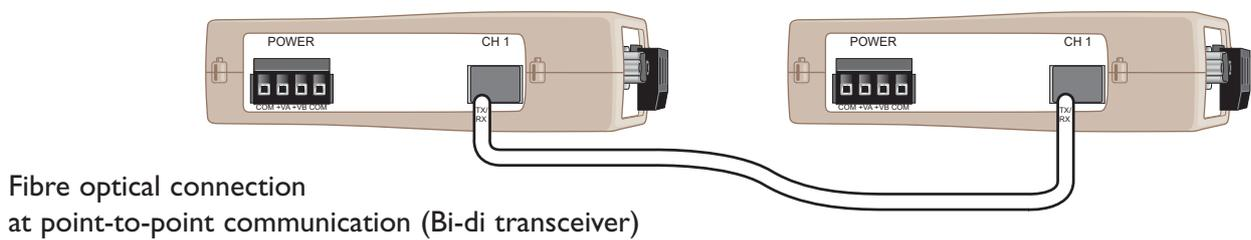
**Note! The bi-di transceivers must always be used in pair, see example:**
