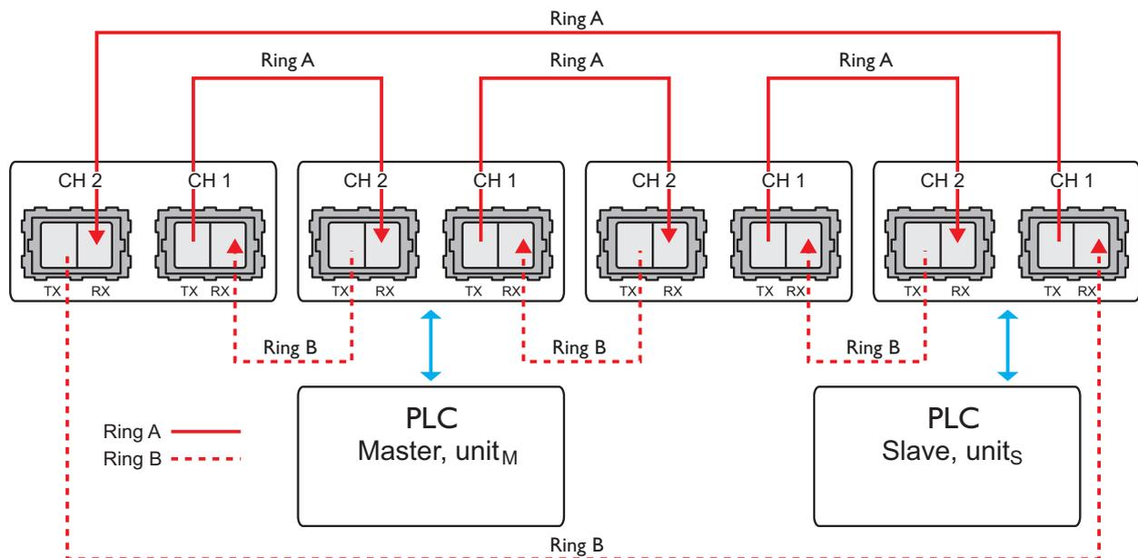
**Note!** Ring A start up at TX (channel 1) and ring B ends up at RX (channel 1).
