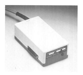
The KM-1A is a converter between 20 mA Current Loop and EIA RS232-C or CCITT V.24 and V.28. The unit can be used when equipment with different interfaces are to be connected.
