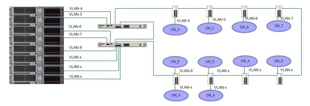
Each DN\_x is a different protocol running in a VLAN In this application all the protocols listed below are running simultaneously over a Gig/b FRNT ring with no loss of performance or timing;
