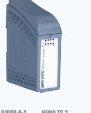
The MCW-211-F1G-T1G is an unmanaged media converter with one SFP fibre port supporting 100 Mbit/s or Gbit Ethernet, and one copper port supporting 10/100 Mbit/s or Gbit Ethernet. It is designed for easy use in heavy duty industrial, maritime and rail trackside applications. The unit supports 802.1Q long packets which allow all standard industrial Ethernet protocols to be used.
