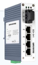
The SDI-541 is a simple and cost effective unmanaged switch suitable for use in a wide range of factory and building automation applications. Two models are available - The SC2 for use on up to 2 km (1.24 mi) of multimode fibre and the SC30 for single-mode applications to 30 km (18.6 mi). A high speed switch core ensures full speed on all ports and transparency to any Ethernet protocol.
