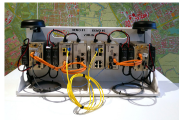
A demonstration unit developed to support system testing and provide visualisation of the data communication infrastructure required to connect the traffic signals at an intersection.
