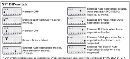
Note! DIP-switch alterations are only effective after a power on.
