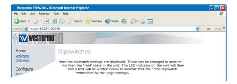
The network interface properties such as speed, duplex and auto-negotiation can be configured by the Web based configuration tool and some settings can be made by hardware DIP-switches.
