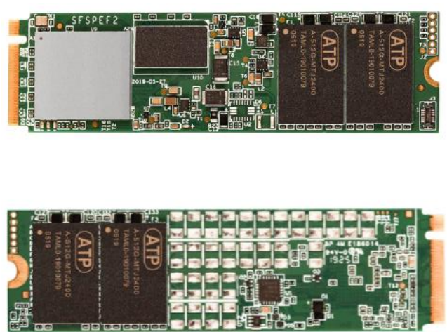
Figure 2 Example M.2 PCIe SSD
