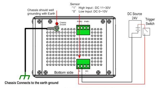
Digital Inputt Wiring simulate Diagram
