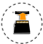
Figure 4. Insertion of micro SD card
