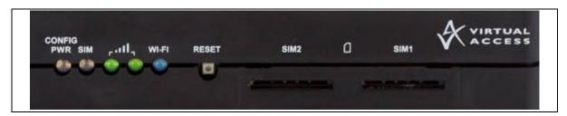
Figure 7: LEDs on the GW1000 Series router
