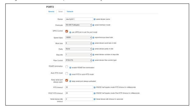
Figure 212: The serial section fields (port mode RS485)
