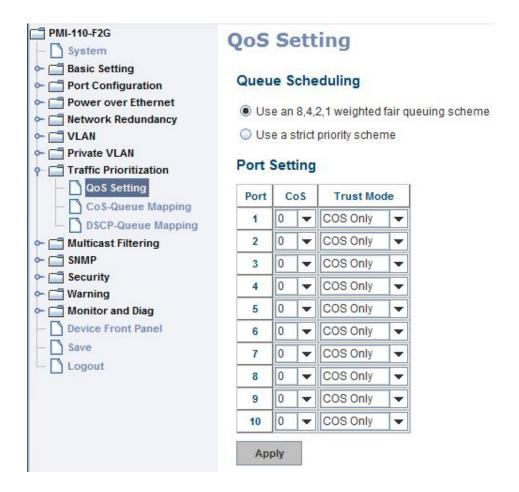
Use an 8,4,2,1 weighted fair queuing scheme. This is also known as WRR (Weight Round Robin). PMI will follow 8:4:2:1 rate to process the packets in a queue from the highest priority to the lowest. For example, the system will process 8 packets with the highest priority in the queue, 4 with middle priority, 2 with low priority, and 1 with the lowest priority at the same time.
