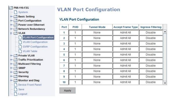
**PVID:** The abbreviation of the **Port VLAN ID**. Enter port VLAN ID here. PVID allows the switches to identify which port belongs to which VLAN. To keep things simple, it is recommended that PVID is equivalent to VLAN IDs.
