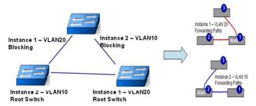
A Common Spanning Tree (CST) interconnects all adjuacent MST regions and acts as a virtual bridge node for communications with STP or RSTP nodes in the global network. MSTP connects all bridges and LAN segments with a single Common and Internal Spanning Tree (CIST). The CIST is formed as a result of the running spanning tree algorithm between switches that support the STP, RSTP, MSTP protocols.
