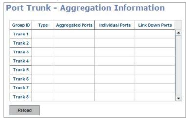
**Group ID:** Display Trunk 1 to Trunk 5 set up in Aggregation Setting.
