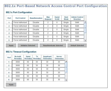
**Port control:** Force Authorized means this port is authorized; the data is free to in/out. Force unauthorized just opposite, the port is blocked. If users want to control this port with Radius Server, please select Auto for port control.
