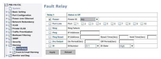
The relay supports multiple event trigger function; click and select type of evnt and setting the detail information, and then click the icon "Apply" to active the replay alarm function.
