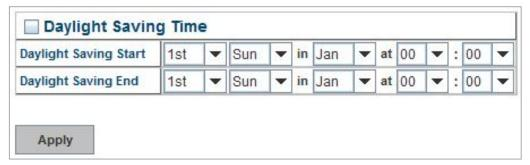
**Daylight Saving Start** and **Daylight Saving End:** the time setting allows user to selects the week that monthly basis, and sets the End and Start time individually.
