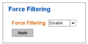
The Force filtering function allows the switch to filter the unknown-multicast data flow. If Force filtering is enabled, all the unknown multicast data will be discarded.
