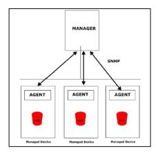
managed switch. An agent translates the local management information from the managed device into a SNMP compatible format. The manager is the console through the network.
