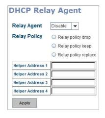
**Helper Address:** there are 4 fields for the DHCP server's IP address. You can fill the field with prefered IP address of DHCP Server, and then click "Apply" to activate the DHCP relay agent function. All the DHCP packets from client will be modified by the policy and forwarded to DHCP server through the gateway port.
