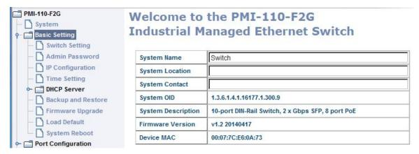
**System Name**: You can assign a name to the device. The available characters you can input is 64. After you configure the name, CLI system will select the first 12 characters as the name in CLI system.
