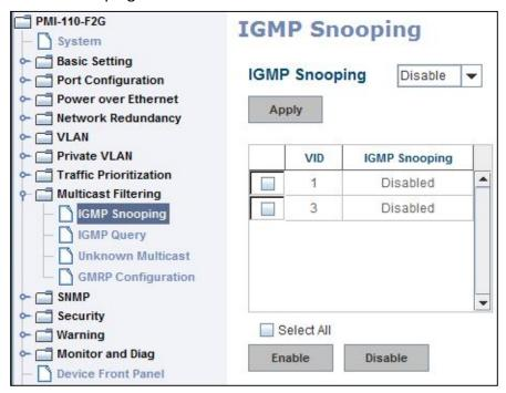
**IGMP Snooping Table**: In the table, you can see multicast group IP address, VLAN ID it belongs to, and member ports of the multicast group. PMI Managed Switch series supports 256 multicast groups. Click on **Reload** to refresh the table.
