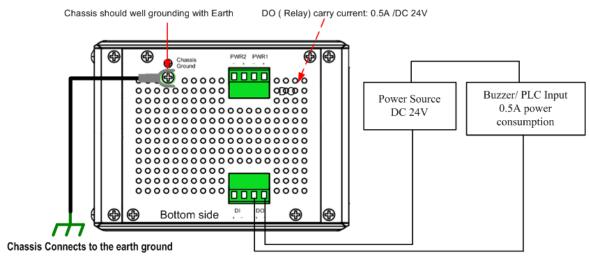
Digital Output Wiring simulate Diagram
