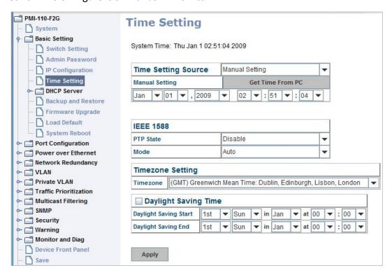
**Manual Setting**: User can select Manual setting to change time as user wants. User also can click the button "Get Time from PC" to get PC's time setting for switch.
