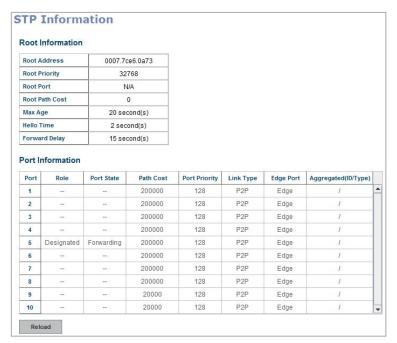
**Port Information:** You can see port Role, Port State, Path Cost, Port Priority, Oper P2P mode, Oper edge port mode and Aggregated (ID/Type).
