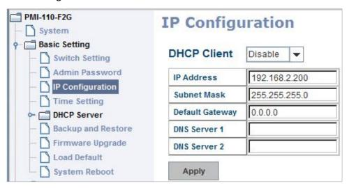
**DHCP Client**: You can select to **Enable** or **Disable** DHCP Client function. When DHCP Client function is enabled, an IP address will be assigned to the switch from the network's DHCP server. In this mode, the default IP address will therefore be replaced by the one assigned by DHCP server. If DHCP Client is disabled, then the IP address that you specified will be used instead.
