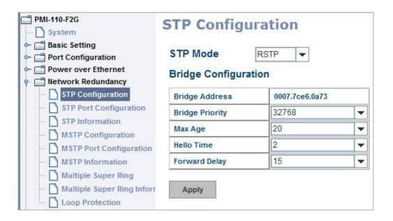
RSTP is the abbreviation of Rapid Spanning Tree Protocol. If a switch has more than one path to a destination, it will lead to message loops that can generate broadcast storms and quickly bog down a network.
