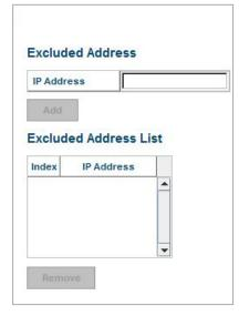
Manual Binding: PMI Switch provides a MAC address and IP address binding and removing function. You can type in the specified IP and MAC address, and then click Add to add a new MAC&IP address binding rule for a specified link partner, like PLC or any device without DHCP client function. To remove from the binding list, just select the rule to remove and click Remove.
