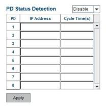
**Cycle time**: user measured the PD system boots duration time. The unit is second. Most of PD system – IP camera will take at least 40~50 seconds. Here, we suggest user sets the cycle time to 90 seconds prevents any wrong suppose.
