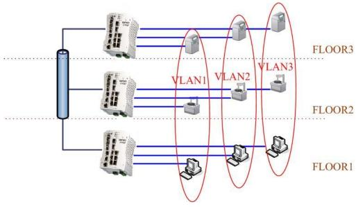
VLAN Configuration group enables you to Add/Remove VLAN, configure port Ingress/Egress parameters and view VLAN table.
